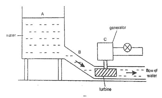
The water turns the blades in the turbine so that electricity is produced by the generator to light up the bulb.
