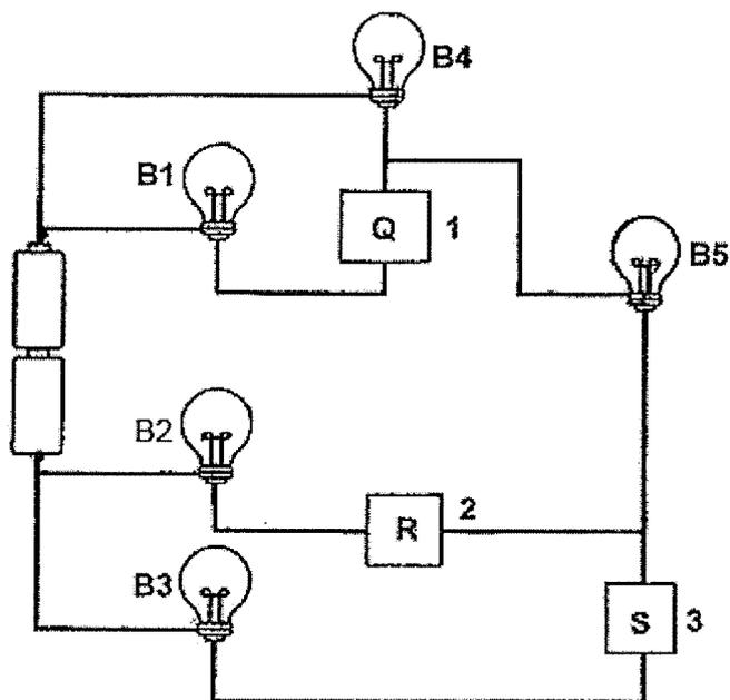
He observed that only bulbs B2, B4 and B5 lit up. He then rearranged the materials S, Q and R and connected to the circuit at positions 1, 2 and 3 respectively.
