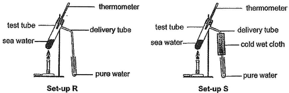
Rahman suggested wrapping the delivery tube with a cold wet cloth, as shown in set-up S, will increase the amount of pure water collected in the test tube over a period of two minutes.
